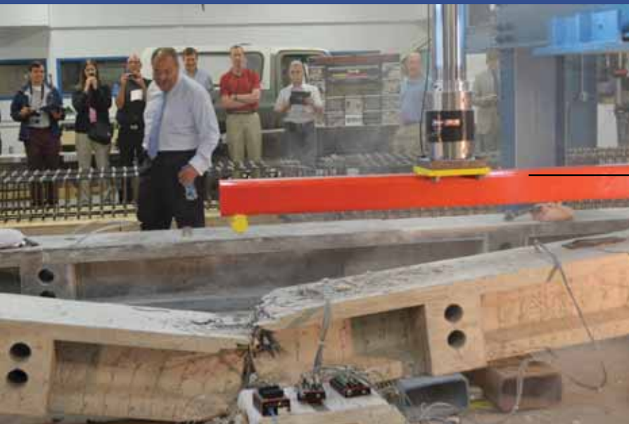
LTU Dean of Engineering Nabil Grace inspects a new type of bridge beam that was tested by applying progressively higher levels of pressure until it failed.
