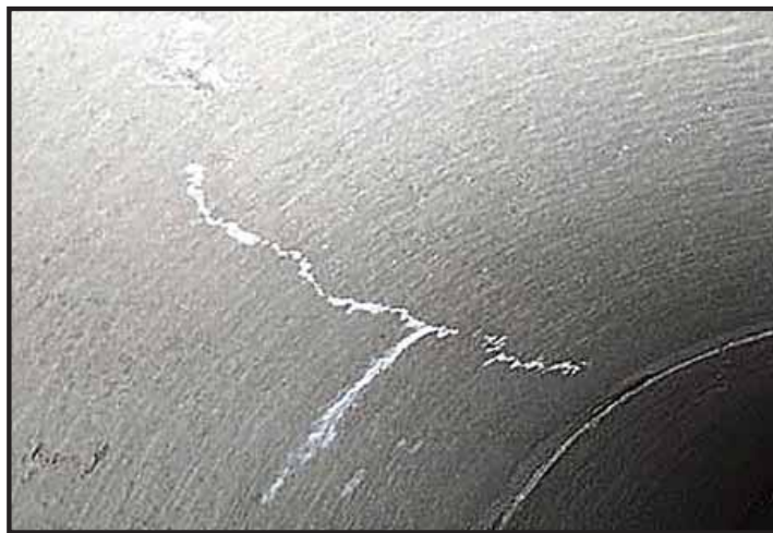
Autogenous healing in concrete pipe.
