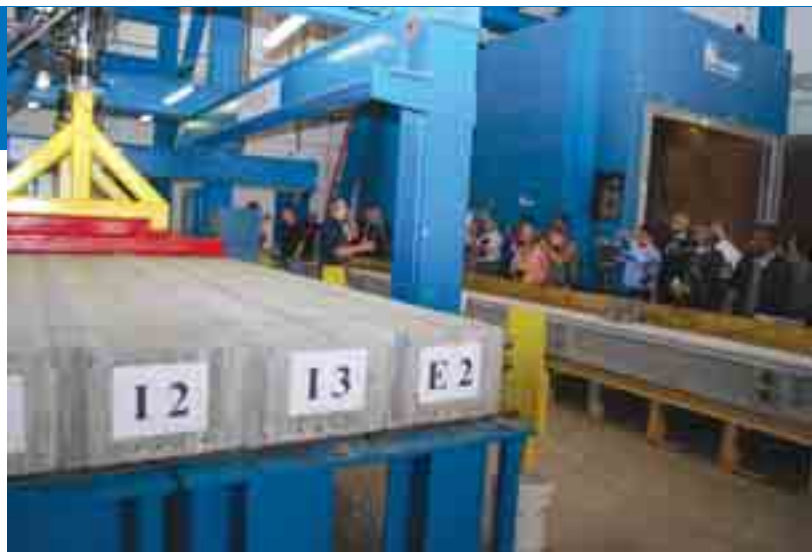
Lawrence Tech Project Engineer Charles Elder describes the process for testing a pre-stressed decked bulb-T beam bridge (in the foreground) to an audience that included government officials and media representatives.
