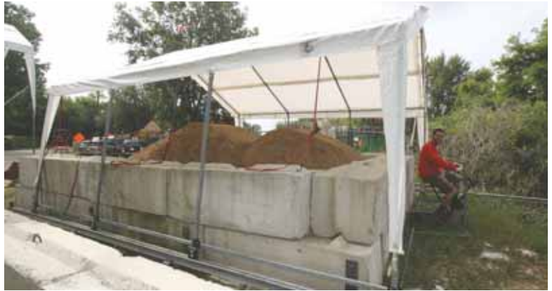
Chris McNeilly proudly displays the invention of a Spartan employee, which allows the tarp to be retracted for reloading of sand that fills sandbags to hold traffic control signs in place within road projects.
