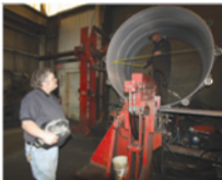
Kevin Pattullo and John Sullivan manufacturing corrugated steel pipe.
