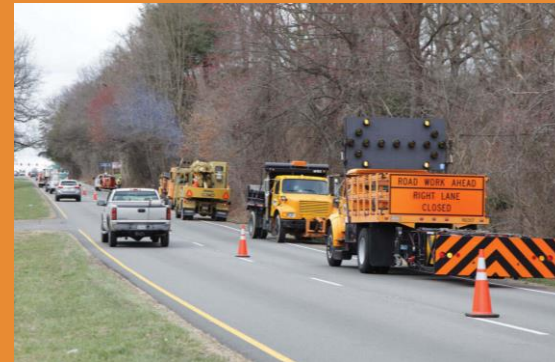
Truck Mounted Attenuators
