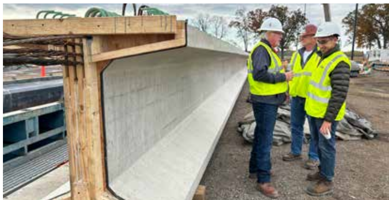
MITA Engineers Jeremiah Leyba and Glenn Bukoski chat with Peninsula Prestress General Manager Dave Marsh next to a large prestressed concrete beam just lifted out of the casting bed.
